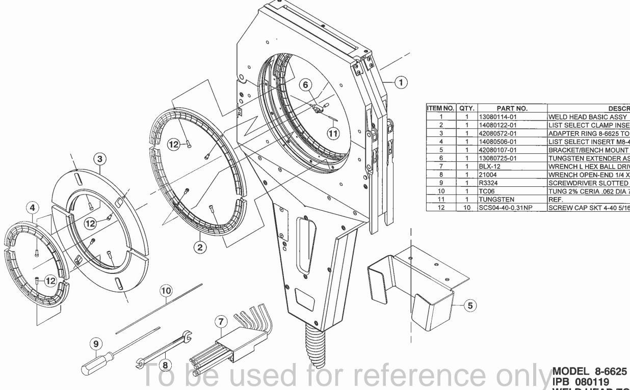
PART NO. **DESCRIPTION** 13080114-01 WELD HEAD BASIC ASSY 14080122-01 LIST SELECT CLAMP INSERT M8-6625 42080572-01 ADAPTER RING 8-6625 TO 8-4000 INSERTS (OPTION) 14080506-01 LIST SELECT INSERT M8-4000 42080107-01 BRACKET/BENCH MOUNT (OPTION) 13080725-01 TUNGSTEN EXTENDER ASSY (OPTION) BLX-12 WRENCH L HEX BALL DRIVE SET 12 PIECE 21004 WRENCH OPEN-END 1/4 X 5/16 R3324 SCREWDRIVER SLOTTED 3/32 X 4IN LONG TC06 TUNG 2% CERIA .062 DIA 7.00L TUNGSTEN REF. 10 SCS04-40-0.31NP SCREW CAP SKT 4-40 5/16 L
